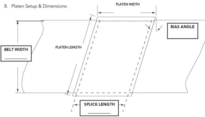
Indicate on the sketch the belt width, splice length and bias angle in the spaces provided. If you require more than one platen set, indicate additional platen dimensions below:
