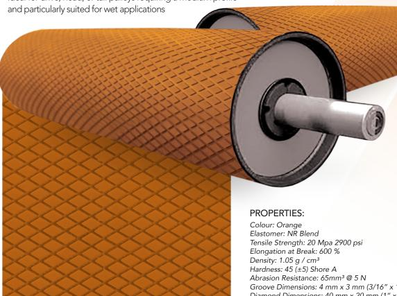
Groove Dimensions: 4 mm x 3 mm (3/16" x 1/8") Diamond Dimensions: 40 mm x 20 mm (1" x 3/4")
