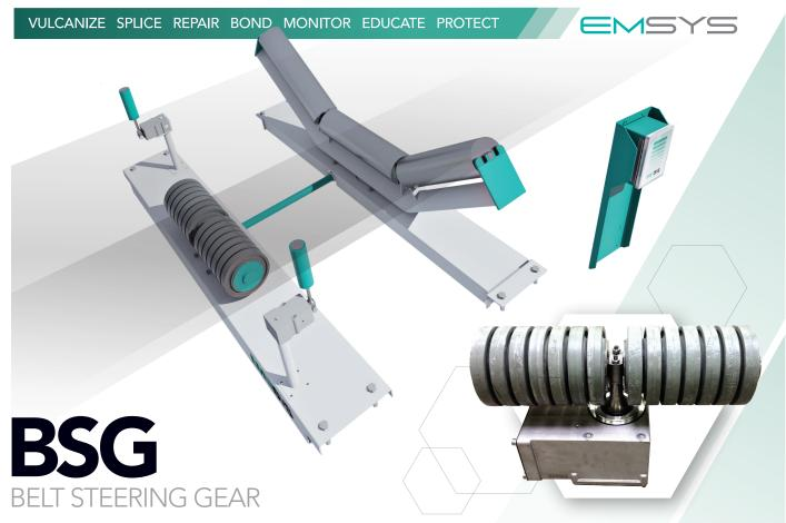
Misalignment or tracking of conveyor belts can lead to material spillage, edge damage, and structural component damages. EMSYS Belt Steering Gear (BSG) utilizes actuators on each side of the conveyor to determine the belts' position and uses a hydraulic cylinder to turn idlers to steer the belt back to its correct position.
